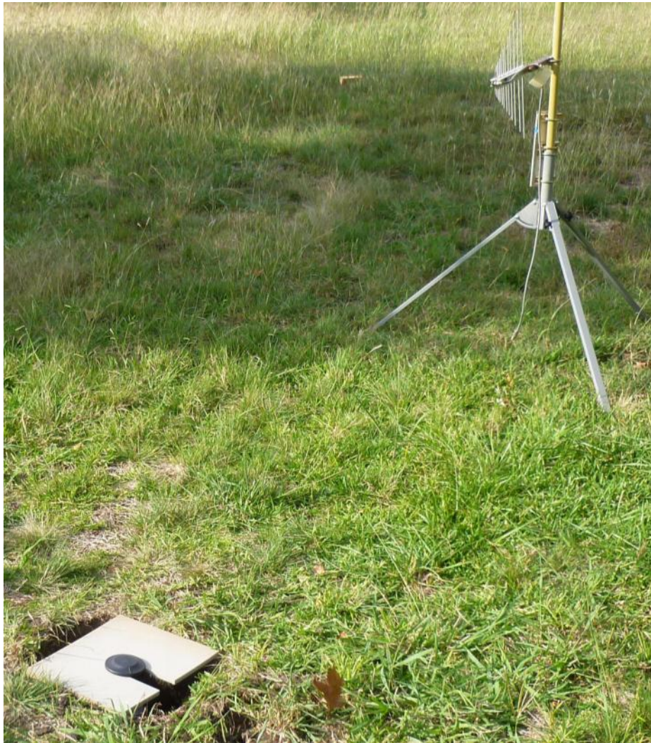
This image shows the test antenna in the right background with the Sensus cast iron pipe cap over the hole in the ground.
